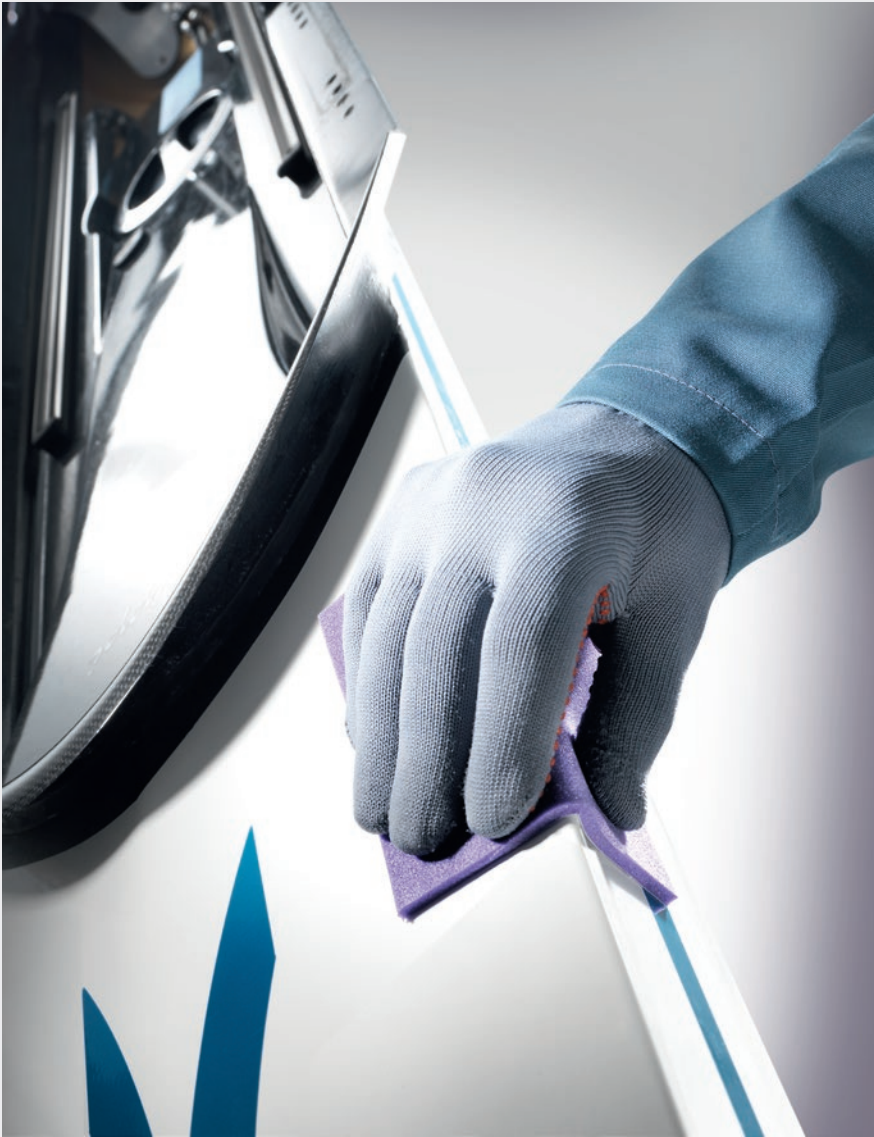
Manual sanding of contours and edges e.g. preparation for painting over painted workpieces, dry sanding
