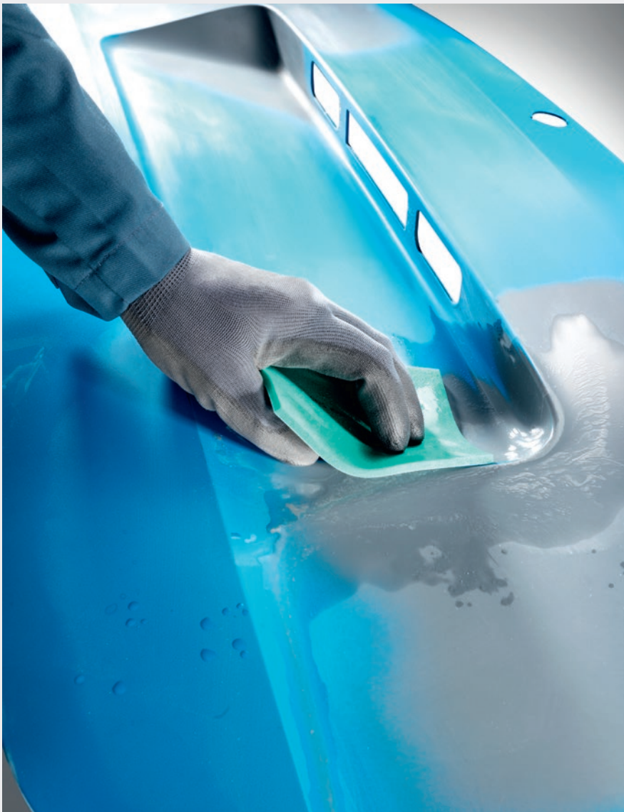
Manual sanding of hard-to-reach areas e.g. wet sanding of paintwork repair spots
