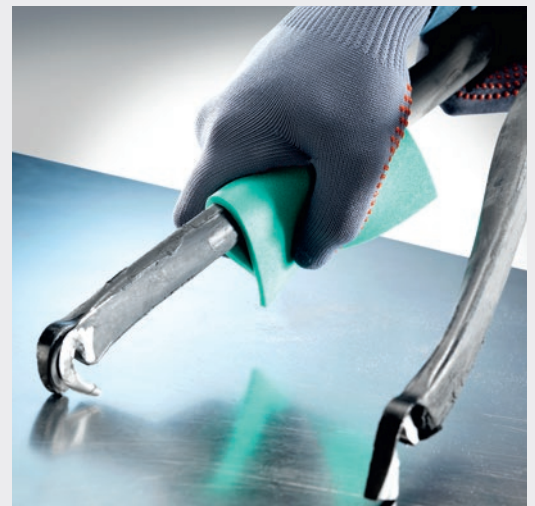
Manual sanding of special shapes e.g. preparation for painting over composites, dry sanding
