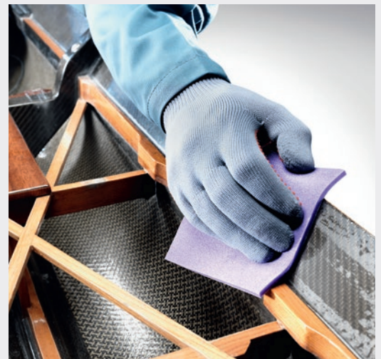
Manual sanding of special shapes and contours e.g. preparation for painting over composites, wet sanding
