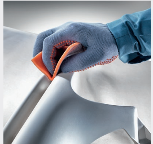
Manual sanding of hard-to-reach areas e.g. keying/sanding out of plastic parts, intermediate sanding of hard-to-reach areas, dry sanding
